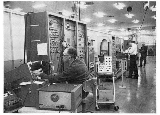
MAINTENANCE, CALIBRATION of QEST and PT testers at the Pantex facility is a precise, demanding job. In this test area, one of many in Sandia's new 20,000 square foot building at Pantex, C. D. Thompson, Mike Zapach, and Del Poer prepare test equipment for forthcoming programs.
